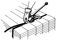
5. Crimp or notch the seal as shown.
