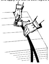
3. While standing to one side of the strap line, tension the strap through continuous up and down motions with the tensioning handle. NOTE: Do not allow the handle to press against the base during the downward portion of the tensioning cycle. This will raise the feedwheel and release the tensioned strap.
