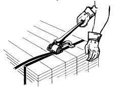
4. Snap a seal on the straps directly in front of the tool, making sure that the seal covers both straps.
