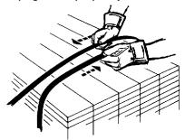
2. Squeeze the tension handle to the base to lift the feedwheel and apply the tool to both layers of strap.
