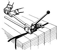
6. Press and hold the handle pawl with thumb. Squeeze the handle to the base and remove the tool from the strap by swinging the rear foot out as illustrated.
